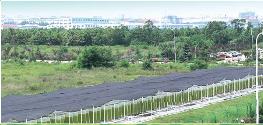
Jülich researchers are comparing different photobioreactors for growing algae. In such a reactor, the nutrient solution drips through fine-mesh sieves together with the algae, enabling them to efficiently absorb light and CO 2 from the ambient air (large picture). In a different reactor, the algae thrive in transparent plastic mats (small picture).
