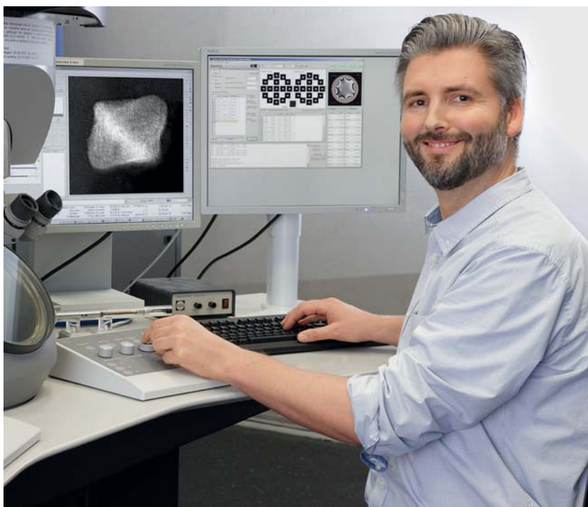
A look at minute details: with the help of an electron microscope, Marc Heggen examines the atomic structure of potential dream catalysts for fuel cells.
